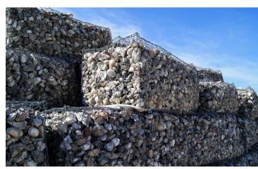
Armourstone from Katholm is produced in accordance with the EN13383-1 standard and comes in three fractions, 45/180, 150/300 and 300/500, although they can of course be adjusted to your specific needs.
